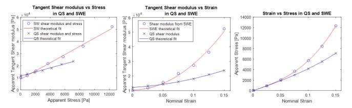
Fig. 4. Nonlinear parameter estimation for a porcine muscle tissue using SWE and QS measurements in 1 mm compression steps (7 steps) using a motorized sensor system with a linear (a), quadratic (b) and third order fit (c).
