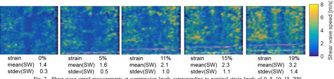
Fig. 2. Shear wave speed measurements at compression levels corresponding to nominal strain levels of 0, 5, 10, 15, 20%
