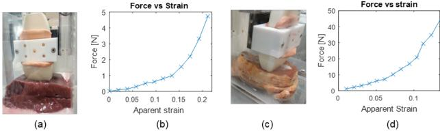
Fig. 1. Experimental setup for liver (a) and muscle (c) with the corresponding force measurement values (b,d).
