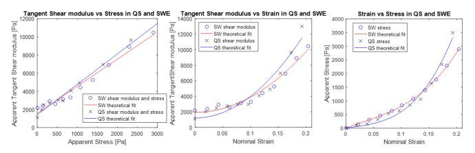
Fig. 3. Nonlinear parameter estimation in ex-vivo liver using CompExp fine compressions of 0.5 mm steps with a motorized system for linear (a), quadratic (b) and third order fit (c) parameters estimated using QS and SW approaches.
